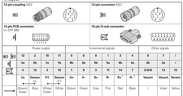
Cable shield connected to housing; UP = Power supply voltage Sensor: The sensor cable is connected to the respective voltage supply in the encoder (ERO 6xxx and ERA in the encoder connector) Vacant pins or wires must not be used.
