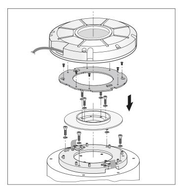
Mounting the ERP 880 (in principle)
