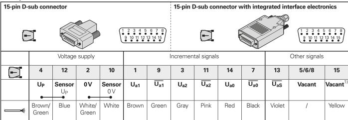
**Cable shield** connected to housing;  $\mathbf{U_P} = \mathsf{Power}$  supply voltage **Sensor:** The sensor cable is connected to the respective voltage supply in the encoder (ERO 6xxx and ERA in the encoder connector) Vacant pins or wires must not be used.
