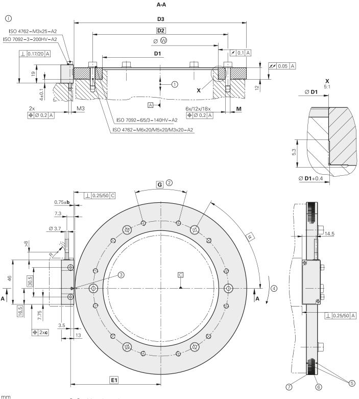
Tolerancing ISO 8015 ISO 2768 - m H ≤ 6 mm: ±0.2 mm
