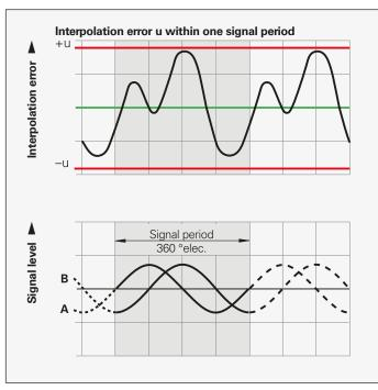
Interpolation errors within one signal period  $\pm u$  is specified in percent of the signal period. For modular angle encoders without integral bearing the value is typically better than  $\pm 1$  % of the signal period (ERP 880:  $\pm 1.5$  %). You will find the specified values in the Specifications.
